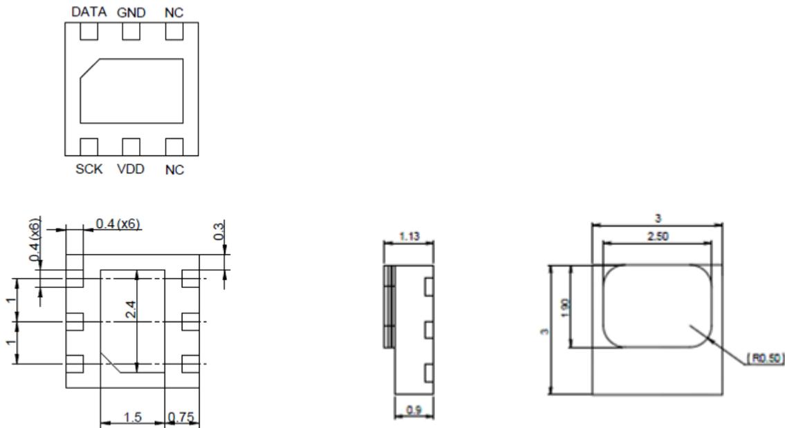
Dimensions are given in mm, tolerances are  $\pm 0.1$  mm. The die pad (thermal center pad) is internally connected to GND.
